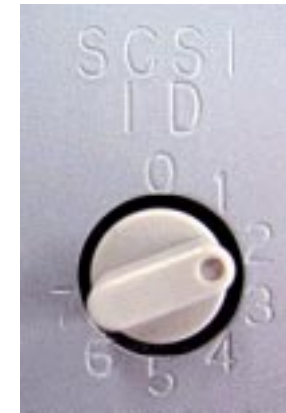
Figure 1-4. SCSI ID Switch
