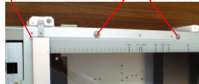
Figure 4-20. Determining the Glass Frame Assembly Position
