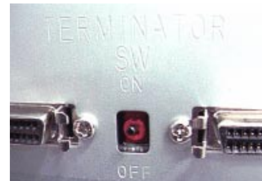
Figure 1-5. SCSI Terminator Switch
